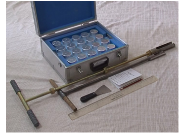
图3 烘干称重法土钻和土盒 Fig. 3 The soil drill and box used in the drying weighing method
