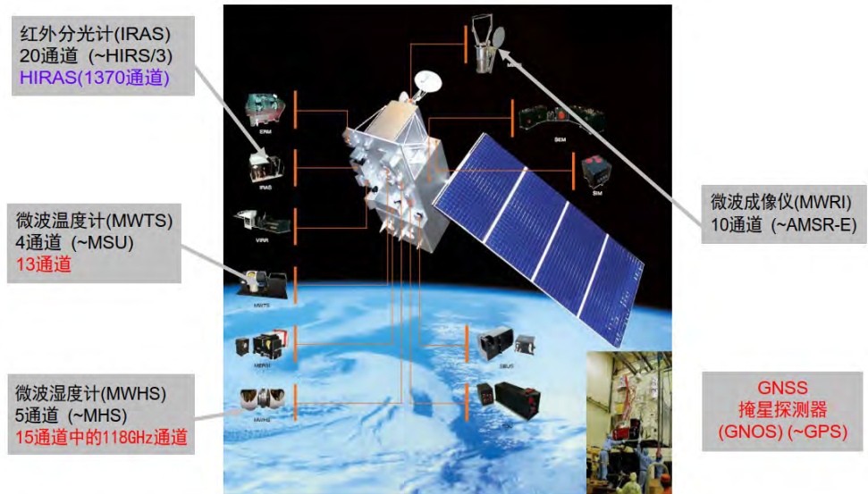
图1 FY-3A/B/C/D用于数值天气预报的探测载荷 [8] Fig.1 The FY-3A/B/C/D instrument suits for NWP
