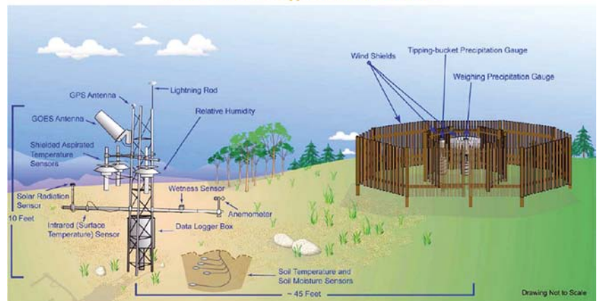
Instruments at a Typical USCRN Station
